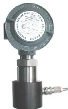
Fig. 2 From this position remove the magnet and the zero calibration procedure is terminated
