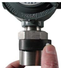
Fig. 2 From this position remove the magnet and the zero calibration procedure is terminated
